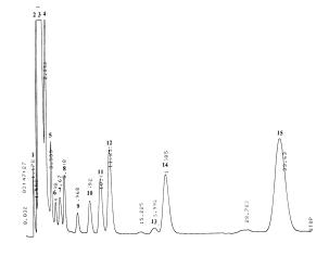
Techcomp is coming up with a "fingerprint" that identifies whether the White Liquor in consideration is safe for human consumption. Techcomp has researched and devised this "fingerprint" (see left), which is actually a chromatogram that accurately identifies the common ingredients in White Liquor.
